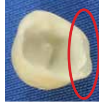
Incorrectly etched (lacking etching on select internal areas and margin edges).
